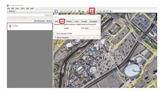
Draw a line by clicking two points across the building site, then tick the checkbox for "show Elevation Profile".
